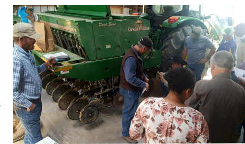
Rex Herring and Steven Sheets demonstrate how to calibrate a no-till drill.
