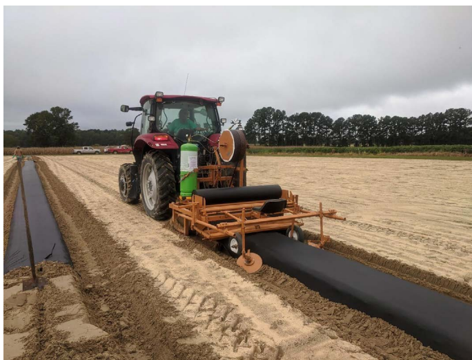
Figure 1-10. A single-row tractor towing a plastic mulch bed shaper with fumigation rig. Beds are pre-bedded through a single pass without plastic and fumigant application, and then followed up by a second pass, during which fumigants are applied and plastic is laid.
