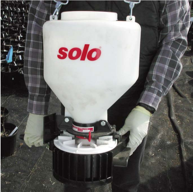
Typical belly-grinder applicator for granular herbicides
