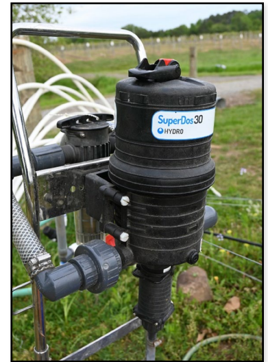
Figure 7: A Dosatron injector pump, a type of positive displacement metering pump.
