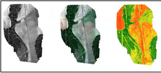
Figure 3. Comparison of single band imagery (NIR) (left), RGB imagery (middle), and calculated NDVI (right) for detecting feral hog damage to a pasture.
