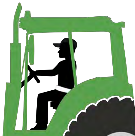
Figure 1. Buckle up if your tractor is equipped with a roll-over protective structure (ROPS).
