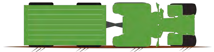
Figure 8. Fishtailing or severe braking at high speed can cause jackknifing and rollover.
