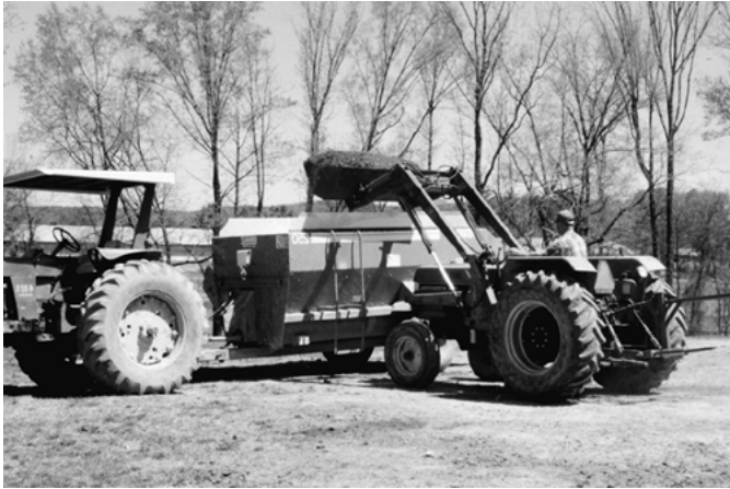
Some cattle producers use front-end loaders and mixer-feeder wagons or feed trucks to aid in mixing and delivering rations containing litter to feed bunks.
