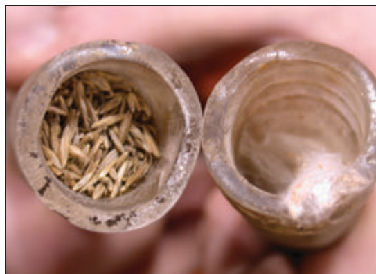
Figure 1. Seed tube on left plugged with old seed from a previous use and tube on right plugged with a spider web. All seed tubes should be checked for obstructions before each use to avoid skipped rows resulting from plugged tubes.
