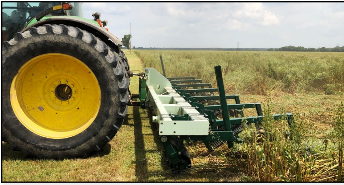
Figure 2. Photo of a roller crimper flattening the standing cover crop into a mat prior to cash crop planting, courtesy of Dr. Bill Robertson, University of Arkansas Cooperative Extension Cotton Agronomist.
