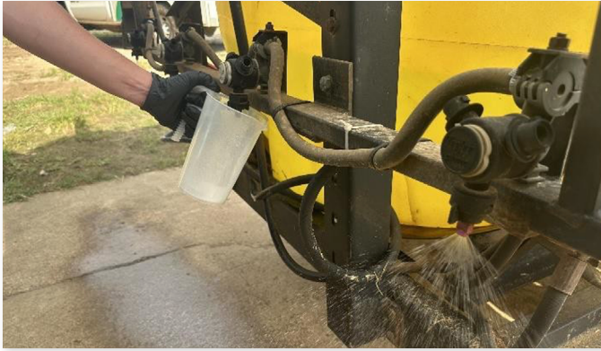
Figure 1. Catch test on a boom nozzle using a catch container.
