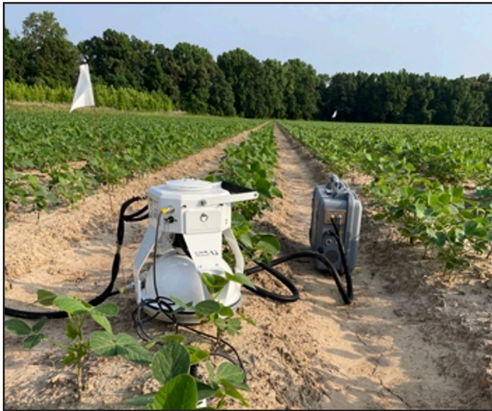
Figure 1. Quantifying soil respiration using absorption spectroscopy equipment in a soybean field near Dumas, AR. Picture taken in 2024.
