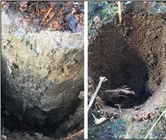
Figure 2. Example of visible difference between a saturated soil (left) and the same soil at field capacity (right). Images are depicting the same Dewitt silt-loam soil (Typic Albaqualf) under different water management regimes.
