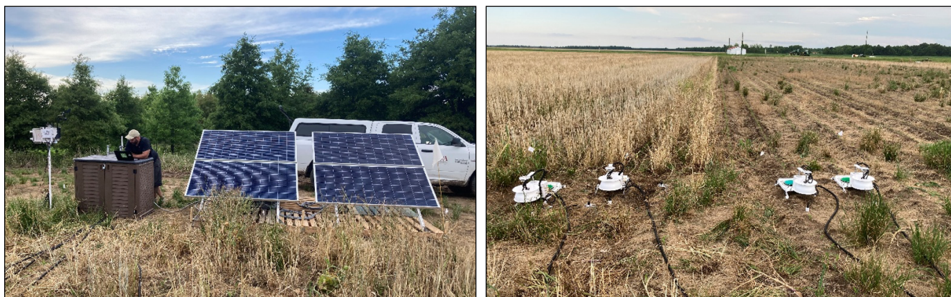
Figure 3. Automated, long-term, flow-through-chamber system with solar power supply (left panel) and four connected sampling chambers (right panel) that stays in the field and simultaneously measures carbon dioxide, methane, and nitrous oxide concentrations multiple times per day. Two chambers are in a cover-crop treatment (right panel, left), while two chambers are in a no-cover-crop treatment (right panel, right).
