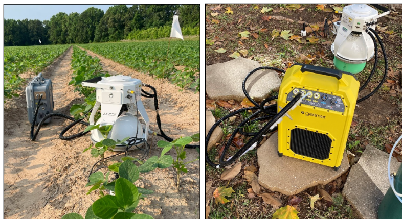
Figure 2. Flow-through chamber and two LI-COR greenhouse gas analyzers (left panel) and a flow-through chamber and a Gaset analyzer (right panel) that simultaneously measure carbon dioxide, methane, and nitrous oxide concentrations in the field.
