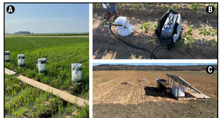
Figure 1. Analytical methods for greenhouse gas measurement. Vented, non-flow-through, closed-chamber method (A); portable, in-field LI-COR carbon dioxide/methane analyzer paired with a LI-COR smart chamber (B); and an automated, semi-permanent LI-COR system paired with LI-COR long-term chambers powered by solar panels (C).
