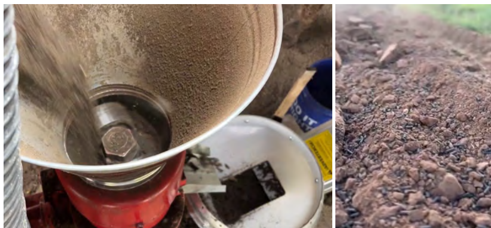
Figure 1. Photo of generation of BAPL with a small pellet machine (left) and BAPL application in the farm field (right)
