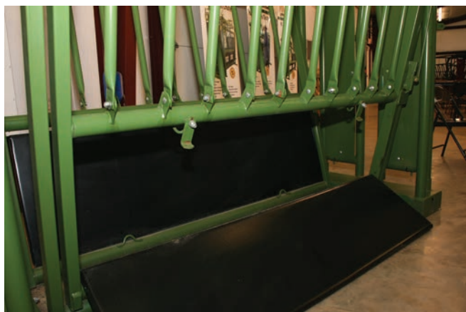
FIGURE 7. Lower panels can be removed to access the cattle's feet and legs.
