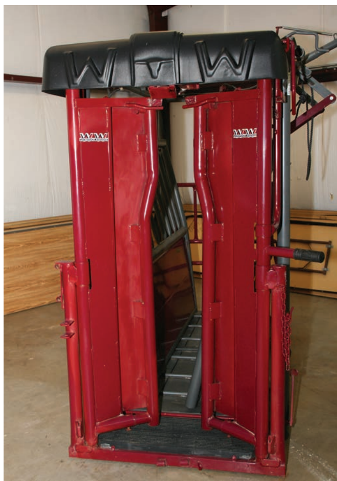
FIGURE 5. All controls are on the front of the chute for one-man operation.
