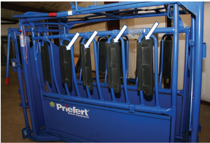
FIGURE 8. Flexible poly blinders to help funnel cattle into the headgate by reducing visual distractions from outside the chute.
