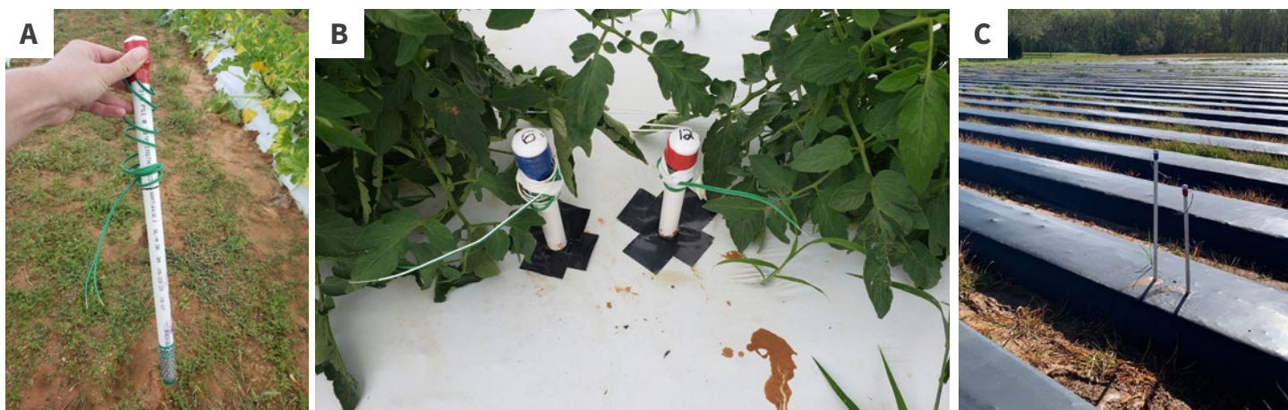
Image 9.8. An example of a soil moisture sensor (A). A tomato planting with one sensor placed 6 inches into the soil and the second at 12 inches (B). Two sensors set up to monitor soil moisture in a strawberry field (C).
