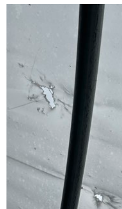
Image 4.16. Hail damage on 6 mil greenhouse grade plastic. A tunnel covered with a woven plastic received no visible damage from the same hailstorm. Images provided by Kyle Manning from Fat Rabbit Farms.
