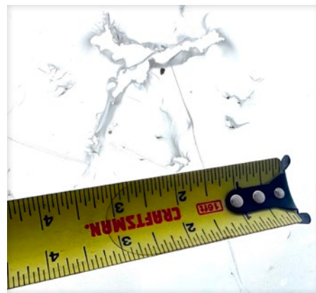
Image 4.16. Hail damage on 6 mil greenhouse grade plastic. A tunnel covered with a woven plastic received no visible damage from the same hailstorm. Images provided by Kyle Manning from Fat Rabbit Farms.
