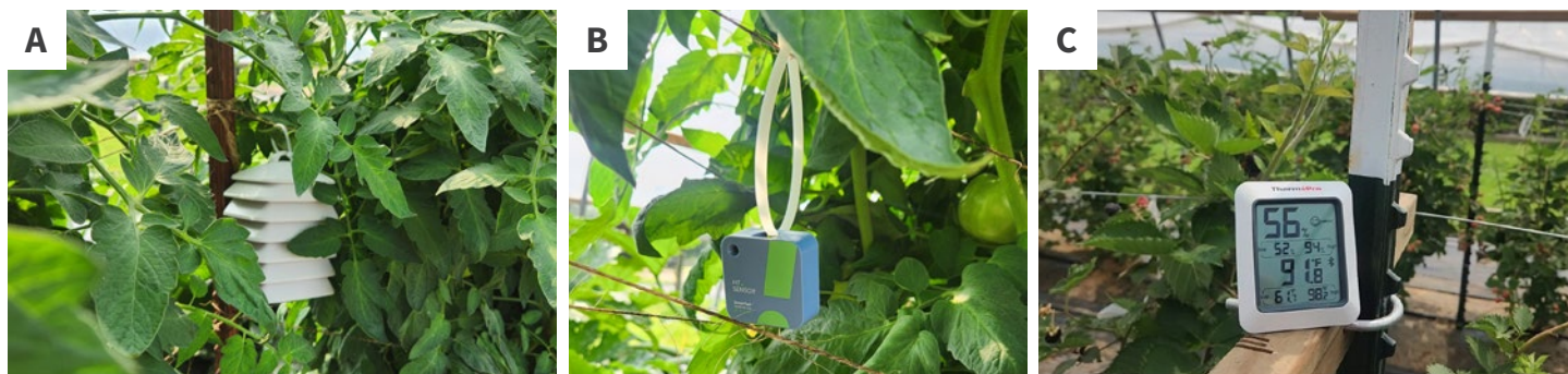
Image 5.17. Examples of different types of temperature and humidity sensors. Sensor complexity can range from loggers that can record climate conditions every minute and connect to a phone or computer (A, B) to sensors that just shows the current conditions and the 24 hour high/low (C). Temperature sensors can be placed inside solar shields to prevent inaccurate temperature readings (A).
